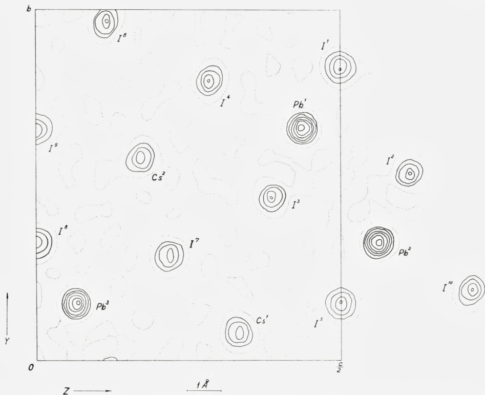
Fig. 2. Electron projection of yellow \text{CsPbI}_3 on the bc -plane. Contour lines are drawn at the relative electron densities 0, 100, 200, 300, 400, 500, and 600.
